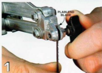
1 Tool-free blade clamping is the way to go. Most tool-free systems use a threaded knob to clamp the end of the blade in place.
