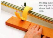
You can square boards and cut them to length without having to flip the stop each time by hand.
