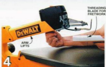
4 You just can't beat the lifting upper arm on the DeWalt for threading blades. Release the blade from the upper holder, lift the arm, thread the workpiece over the blade, lower the arm, reattach the blade and you're ready to go.
